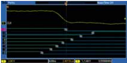
Output of DAC Signal) Notice how FilterVu™ clearly shows the noise-free steps of the DAC in the foreground trace (yellow) which has removed all frequencies above 5.5 kHz. FilterVu also captures and displays high-frequency glitches up to the full bandwidth of the oscilloscope in the background trace (orange).
