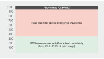
Figure 1- Measurement Ranges with rated range reference
