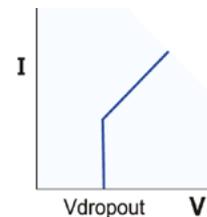
Resistive discharge (conductance mode) with voltage dropout.
