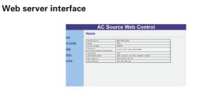
Built-in web server that allows users to configure, control, or monitor the basic settings of the power source from a remote computer using a web browser.
