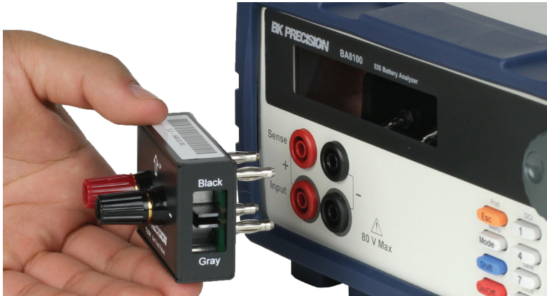
TLC81 plugged-in to the front panel
