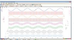
thmetic, logarithmic, trigonometric and other functions. Define a function using the push-button control panel or type an equation in the text box. **PicoScope:** the display can be as simple or as complex as you need. Begin with a single view of one channel, and then expand the display to include any number of live channels, math channels and reference waveforms.
