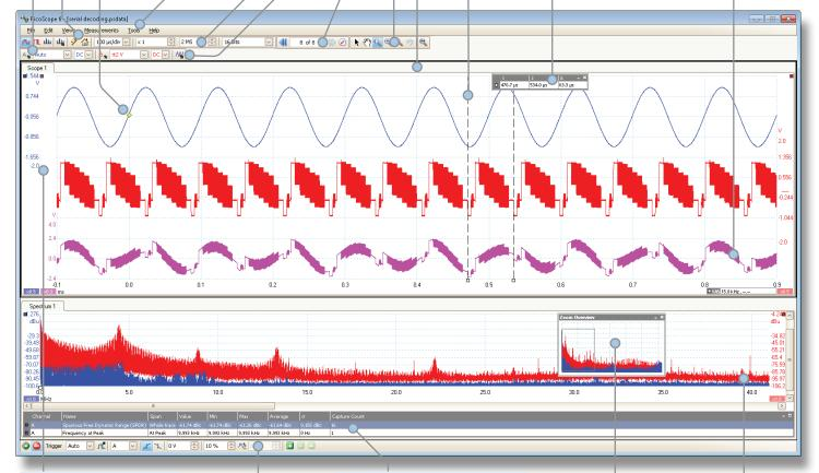
**Movable axes:** The vertical axes can be dragged up and down. This feature is particularly useful when one waveform is obscuring another. There's also an **Auto Arrange Axes** command.
