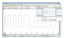
To help you find you way around the buffer memory, you can divide it into as many as 10,000 individually triggered segments. Use the visual buffer navigator to scan through the segments, or set up a mask to filter out the waveforms of interest.
