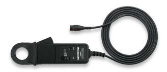
This AC/DC current probe is used to measure currents from 100mA to 1000A over a broad frequency range. The measurement principle is based on the Hall Effect that registers the magnetic field generated by the current flow. Even for complex waveforms a high degree of measurement accuracy is achieved. The output voltage is proportional to the measured current and well suited to be displayed on an oscilloscope. The current probe complies with the safety standards defined in IEC/EN 61010.
