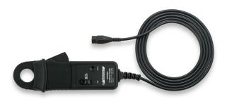
This AC/DC current probe is used to measure currents from 1mA to 30A over a broad frequency range. The measurement principle is based on the Hall Effect that registers the magnetic field generated by the current flow. Even for complex waveforms a high degree of measurement accuracy is achieved. The output voltage is proportional to the measured current and well suited to be displayed on an oscilloscope. The current probe complies with the safety standards defined in IEC/EN 61010.
