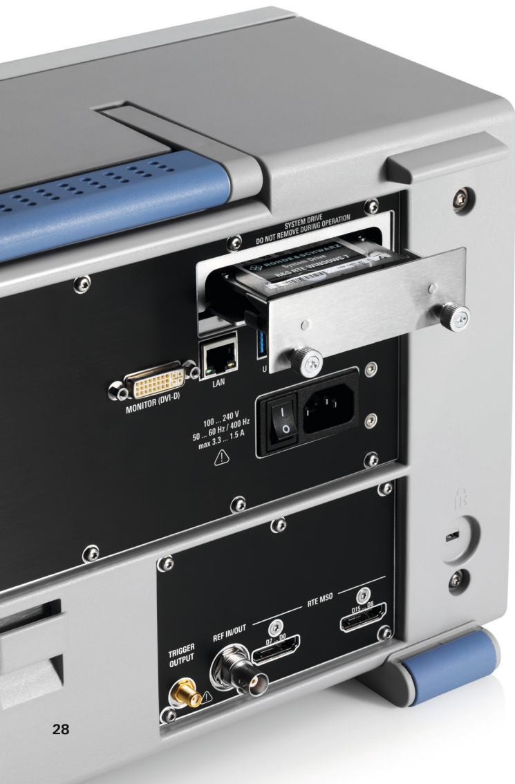
The R&S® RTE SSD can be removed without any tools.
