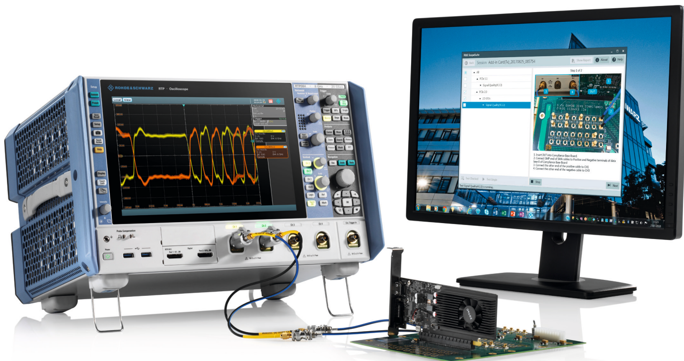
Automated PCI Express compliance test.
