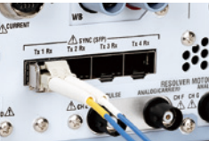
The main unit and sub-units are connected using optical fiber cables and optical transceiver modules.
