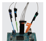
Example of logic probe connection
