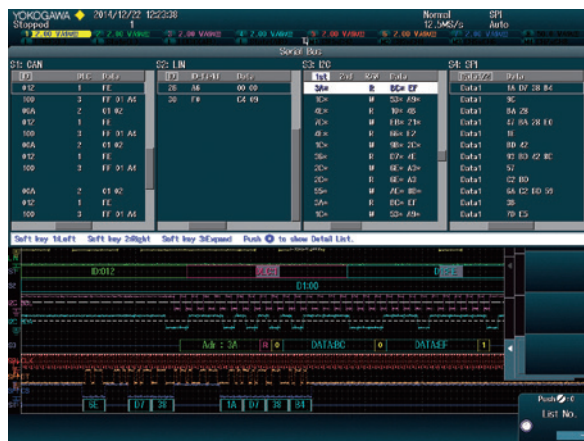
Four bus decode and list display
