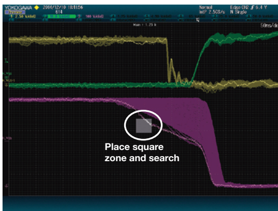
Searching for waveforms that pass through or do not pass through a rectangular zone placed on screen.
