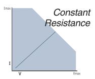
Constant resistance mode simulates a standard resistive load by providing a current drain proportional to voltage. Settings are displayed in Ohms or milli-Ohms.
