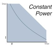
Constant power mode simulates a load whose power consumption is independent of the applied voltage. This is true of many types of equipment that incoporate switchmode regulators.
