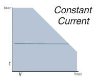
Constant current mode is used for load testing of normal voltage-source power supplies and for constant current discharge testing of batteries.
