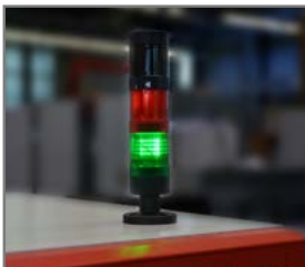
Program sequence display using indicator lamps
