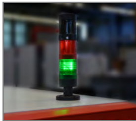
Program sequence display using indicator lamps
