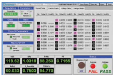
IEC 61000-3-2 Current Harmonics Test (Pre-compliance)
