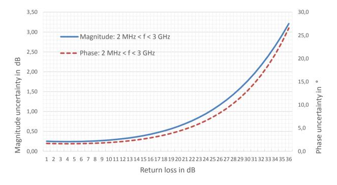
Uncertainty of reflection measurements with the R&S<sup>®</sup>ZN-Z103 calibration unit; temperature: +18 °C to +25 °C, RBW: 10 Hz, power: –10 dBm.
