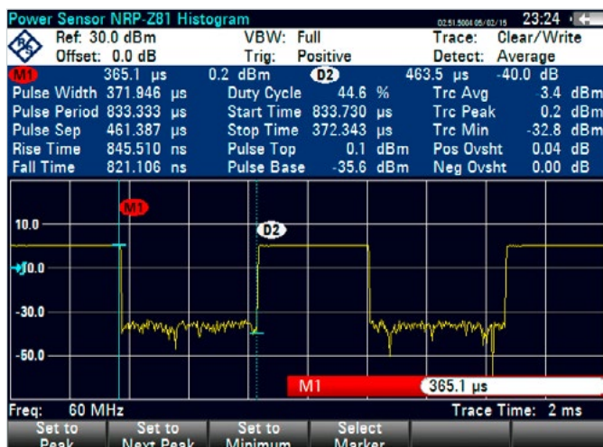
Pulse analysis with R&S FSH-K29 and R&S NRP-Z81 wideband power sensors.
