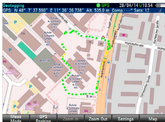
Geotagging results display with R&S®FSH-K16.
