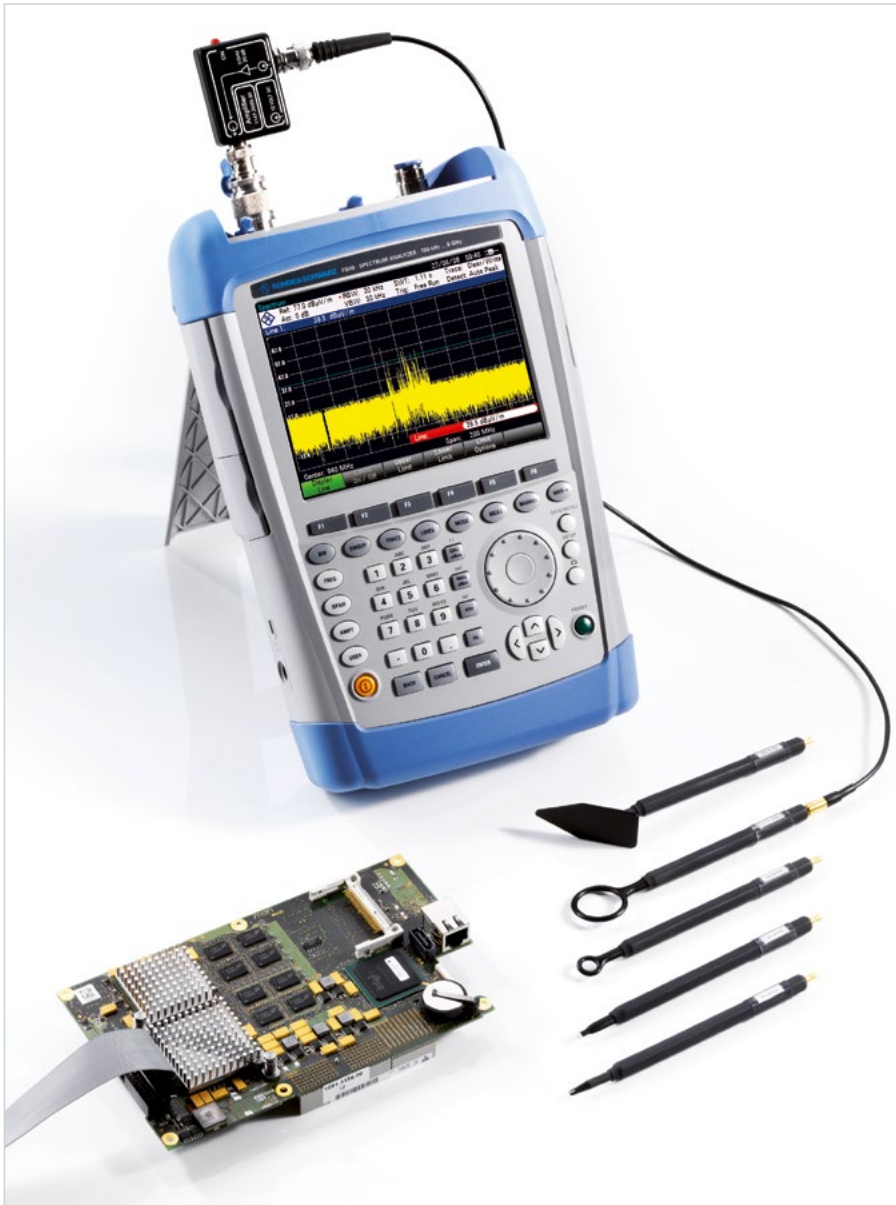
The R&S®FSH with near-field probes and DUT.
