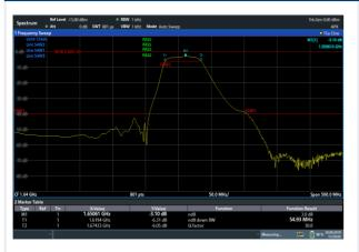
For easy filter qualification, simply define your limit lines for filter characterization, use the n-dB down function to determine the 3 dB points and save the result as a transducer factor
