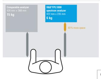
The R&S°FPL1000 with R&S°FPL1-B9 takes up 40 % less space than comparable analyzers on a typical 80 cm workbench.
