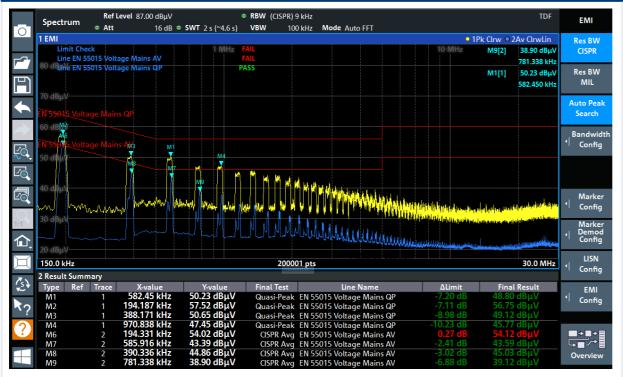
Two detectors are used for the sweep: positive peak (yellow curve) and average (blue curve). Pass/fail information is given according to the defined limits (red lines). The identified maxima ("Auto Peak Search") are automatically measured using the related CISPR detectors (quasi-peak and average) and listed in the results table. The final pass/fail status is clearly shown. The R&S\*FPL applies the correction values (transducer factor) of the used LISN to the measurement results.
