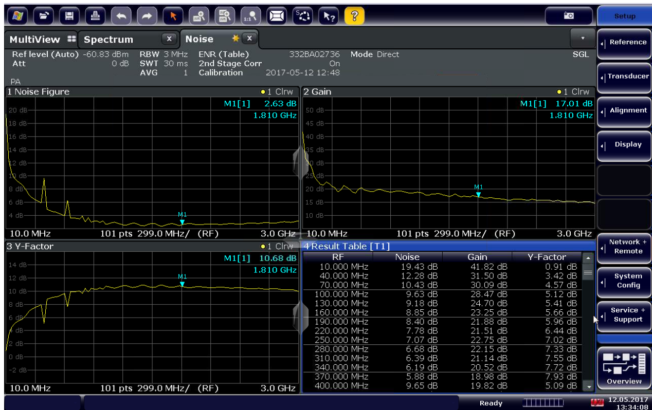
Simultaneous view of graphs for noise figure, gain and Y factor versus frequency and a table of the results in numerical format
