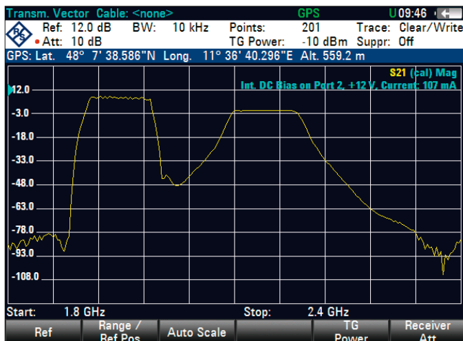
TMA transmission measurement: built-in voltage supply, current measurement, R&S®HA-Z240 GPS receiver connected.
