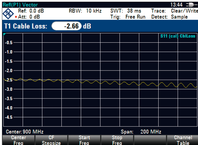
One-port cable loss measurement.
