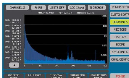
Additionally, eight harmonics can be selected for numeric display of amplitude and phase by touching the harmonic bar of interest. The user may also import harmonic limits, which when enabled will show out of tolerance harmonics in red above the limit line.
