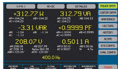
data results (Whr) can also be controlled and viewed from the power data screen. For users with unique data requirements, custom data screens can be built with a spreadsheet application and downloaded to the PA900 via interface or USB drive.
