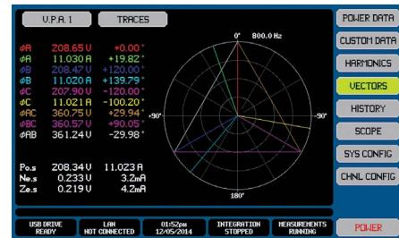
non-measured neutral phase vectors are displayed. The user may enable the display of and select the color of each vector up to a maximum of 10.
