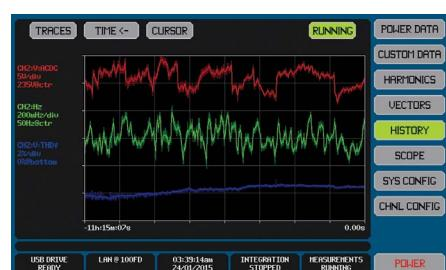
The PA900 automatically maintains a continuous historical record of all non-harmonic measurement results and selected harmonics. Up to four user selectable parameters can be graphically displayed using the HISTORY screen. The user can display the entire recorded period up to 397 days or zoom in as far as 1/64th of the total span. This provides an almost unlimited ability to amplitude zoom and includes a cursor which may be moved throughout the period with a touch of the screen.
