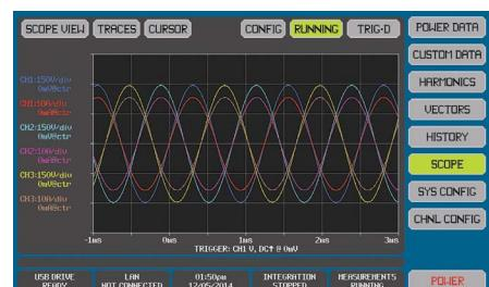
user selectable scaling, offset and color. Timebase, trigger and trigger position are all user selectable. However, with amplitude accuracies as high as 0.03% - you are unlikely to find any other scope with this high level of precision.
