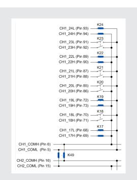
Embedded virtual schematic control simplifies setup and debugging; allows all relays to be engaged independent of application software and device drivers.
