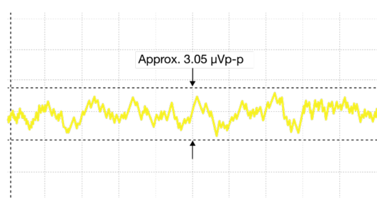
Noise waveform example at 0V output in 10 V output range (observed using a 1000 times amplifier with a 10 kHz band-limiting filter)
