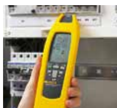
Location of fuses/breakers and assignment to circuits
