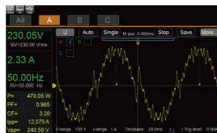
IT7800E built-in Scope function, monitoring DUT waveform in real-time
