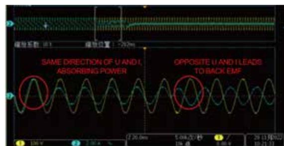
IIT7900P simulates the motor from loading to generating back EMF
