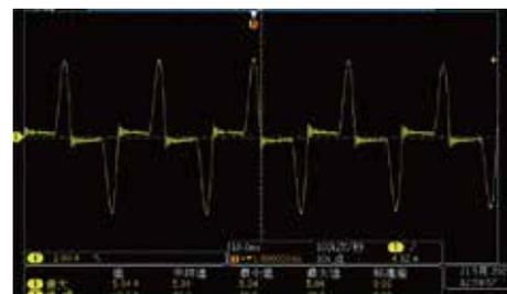
Current waveform of a small AC motor( CF=2 )
