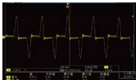
Current waveform of a small AC motor( CF=2 )
