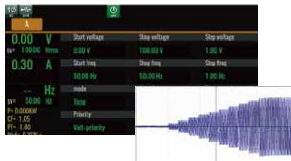
The voltage rises step by step after setting sweep
