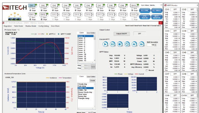
Multi-channel MPPT test
