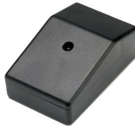
PP066 REED SWITCH Used to detect the presence of a magnetic field such as from a bar magnet or an electromagnet. Alternatively, a simple external switch can be wired to the internal screw terminals. It has a fast response time of 2 ms so can be used as an alternative to a light gate for timing applications.
