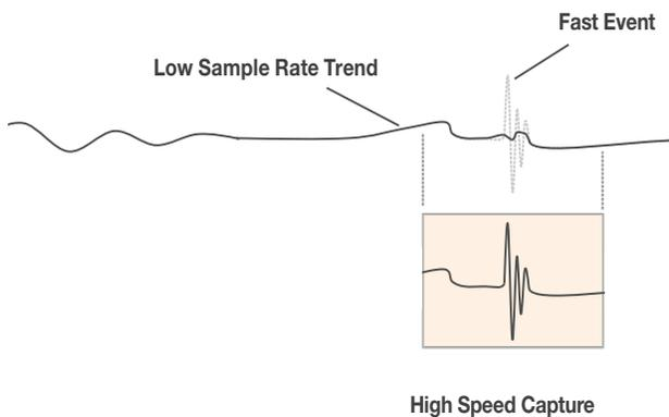
As an example, it is possible to set waveform triggers and capture 5000 high-speed transient events at 100 MS/s while at the same time continuously recording a trend measurement at 10 kS/s for 10 hours.
